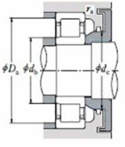
High quality cylindrical roller bearing with machined brass cage from the leading manufacturer TIMKEN. Featuring the TIMKEN EMA design. A premium land-riding cage, unique internal geometries, enhanced surface finishes and a compact design. All this adds up to longer life, improved uptime and reduced maintenance costs.
